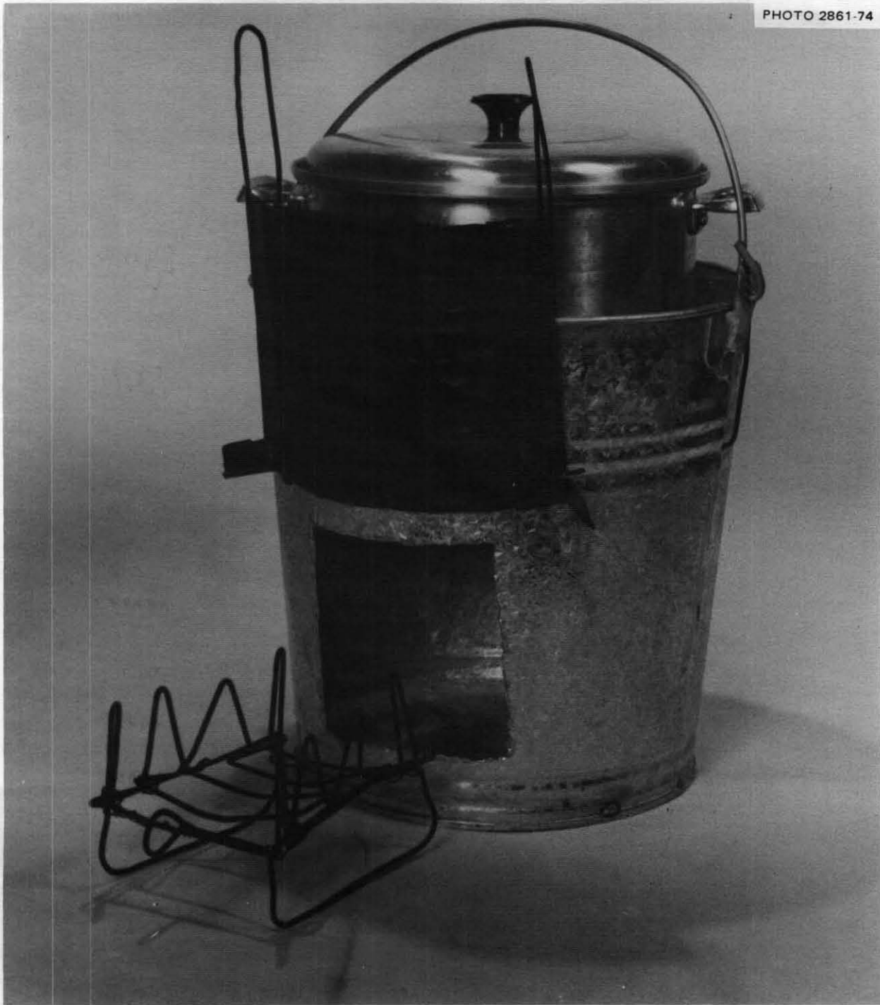
Fig. 37a. Expedient Bucket-Stove, made of a bucket, coat-hanger wire, about 2 ft of finer wire, and metal from an ordinary juice can. This is the most efficient expedient stove tested to date.
